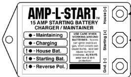
**HOUSE [+]** : This stud is connected to the positive terminal on your house battery(s). Use stranded automotive-grade wire, 12 gauge or thicker (10 gauge if the wire length exceeds 5 feet).
